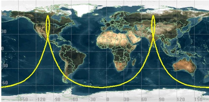
Figure 1: Sub satellite ground track of a Molniya satellite.
