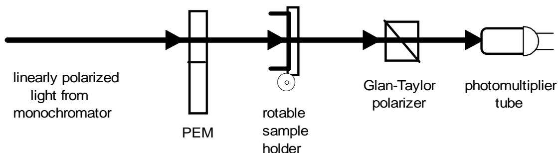
Much care has been put in the selection of the best quality components and a more sophisticated phases-locked loop (PLL) PEM drive has been adopted to reduce voltage applied while improving stability.
