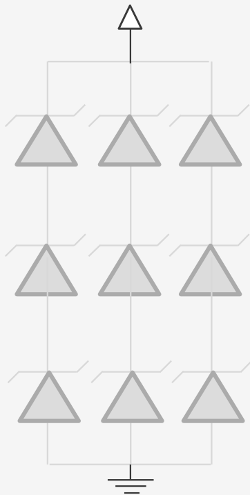
Diodes bridge for 63V clamping schematic
