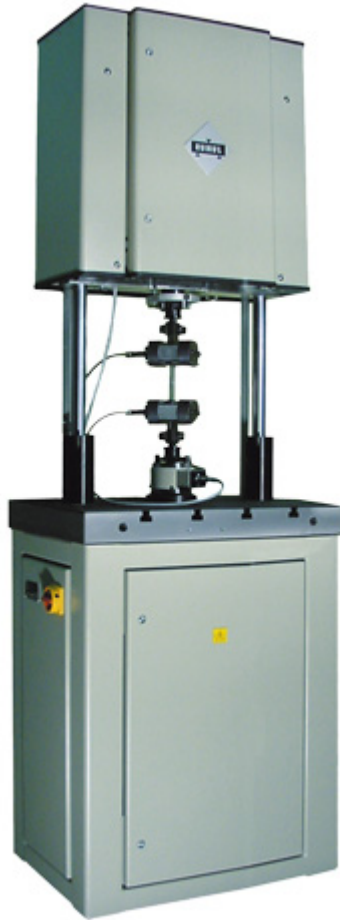
Resonance based Push-pull fatigue testing machine 100-150 Hz Ex.: RUMUL
