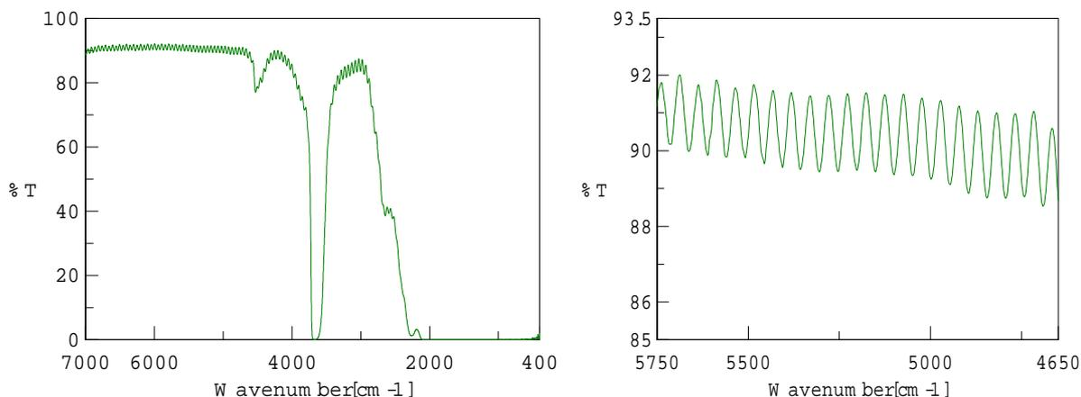
Here we used the film thickness software provided with this IR (as in most of current FT/IR units), so it was easy to calculate the exact path of 97.835  $\mu\text{m}$ , i.e. over 2% less than what stated. It's expected that shorter path cells will show even larger relative errors.
